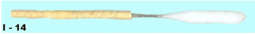
Stuffing fork with a “Q-tip” of stuffing on it, ready to stuff a finger
