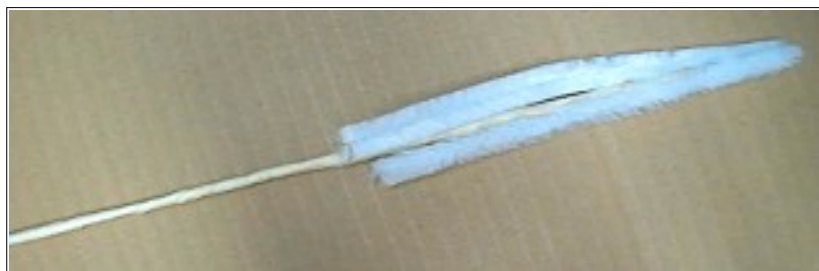
A stuffing fork with a chenille stem hooked in the fork, ready to be guided into a finger.
