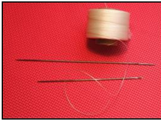
Jointing needles that I use. Either single or double point work. My double point needle is 8" long. The single point needle is 6" long.
